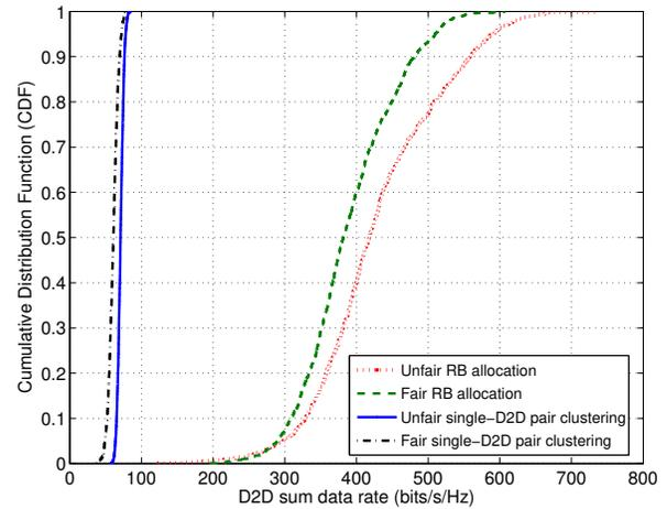
Fig. 2. Comparison of D2D sum data rates
