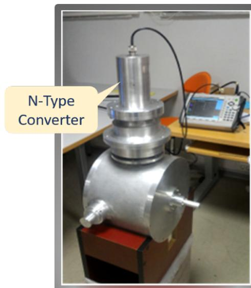
Figure 4.2. Reflection type measurement setup
