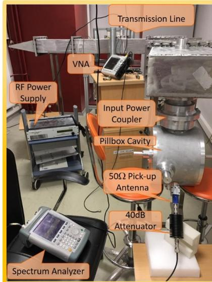
Figure 4.21. Power measurement test stand of the whole system.
