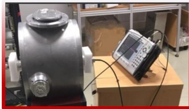
Figure 4.9. Experimental setup 1 with pick-up antennas
