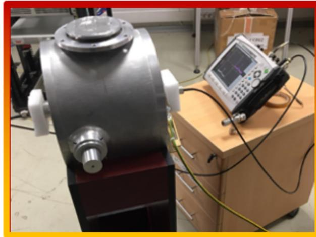
Figure 4.17. Loaded quality factor measurement setup 5 with pick-up antennas
