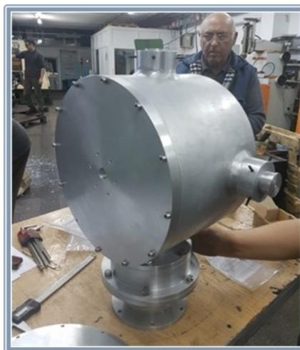
Figure 3.18. The picture of the produced cavity and coupler
