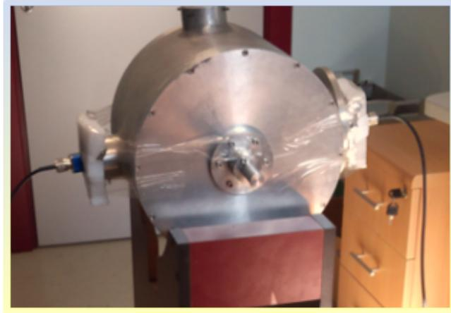
Figure 4.11. Experimental setup 2 with  $50\Omega$  loop antennas.
