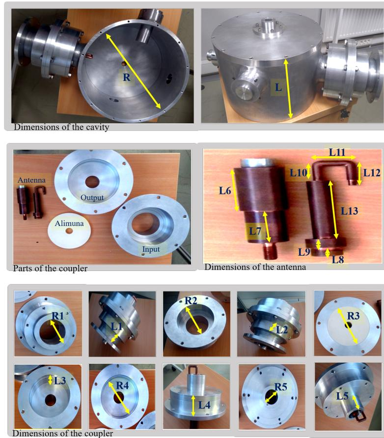
Figure 3.19. Photograph of dimensions of the whole structure
