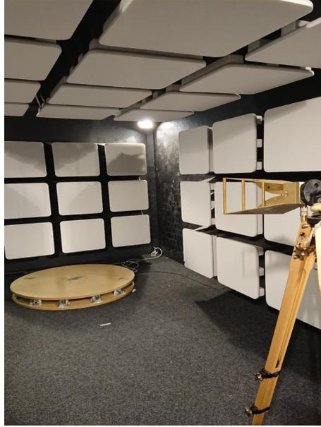
Figure 3.18. Anechoic chamber in IZTECH Laboratories
