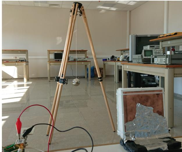
Figure 4.5. The pendulum setup for velocity verification
