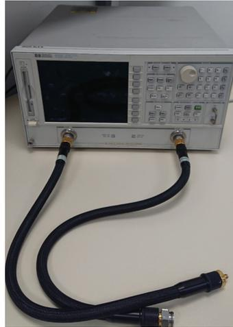
Figure 3.17. Agilent 8720D vector network analyzer
