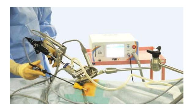
Figure 2.8. Voice Commanded Viky Endoscope Positioner (Source: Takahashi et al. (2017)))
