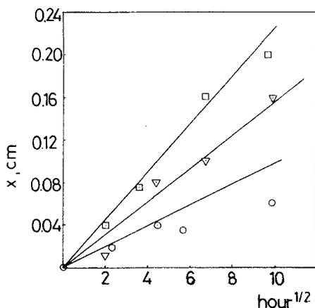
FIG. 7 Colored region thickness ( $x$ ) versus square root of time for thick pellets having 0.10 (□), 0.16 (▽), and 0.30 (○) volume fractions of zeolites.
