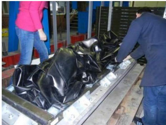
Figure 4.5. Placement of the Rubber Membrane
