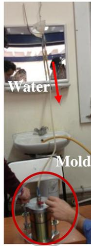
Figure 6.5. Permeability Test Setup
