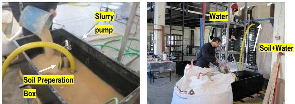
Figure 6.7. Hydraulic Filling Process
