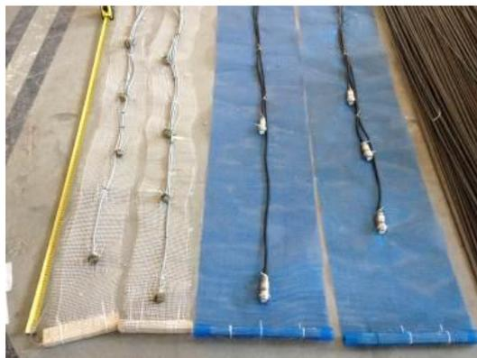
Figure 4.9. Submersible Accelerometers and Pore Water Pressure Transducers Tied on Nets
