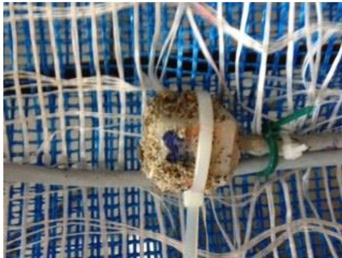
Figure 4.6. Submersible Accelerometer Used in the Shaking Table Test
