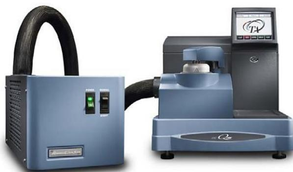
Figure 2.13. The TA Instruments Q10 DSC Device.
