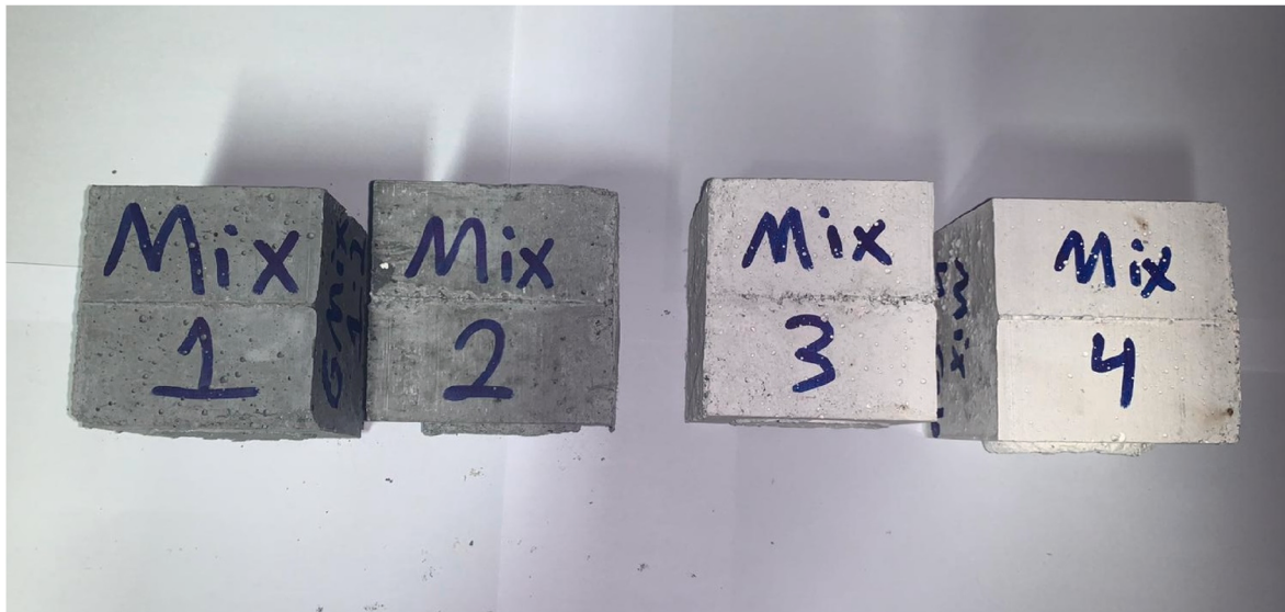
Fig. 2. Photo showing the appearance of samples of the geopolymer mixtures used for ultrasonic pulse velocity (UPV) testing.
