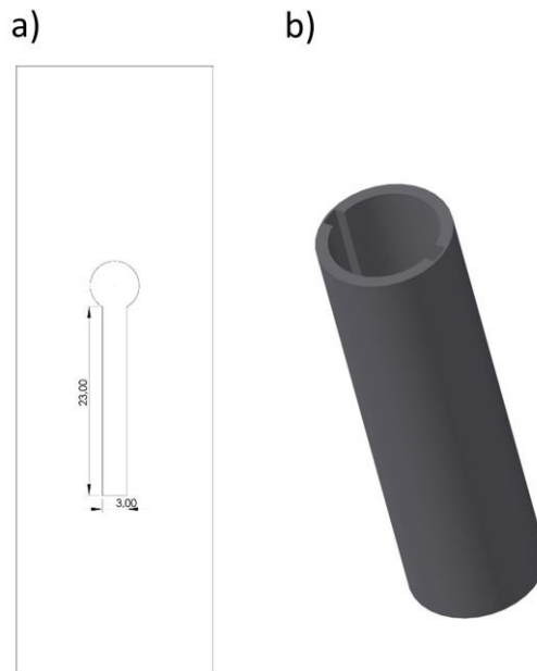
Figure 4.1. The design of Spinochip for blood sample manipulation. (a) A straight channel with a 23 mm length, 3 mm width and 0.15 mm height. (b) A tube suitable for the centrifuge device for the Spinochip
