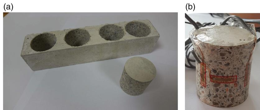
**FIGURE 1** The picture of (a) a core-drilled moulded prismatic concrete plate and a compression test specimen and (b) a strain-gaged quasi-static test specimen
